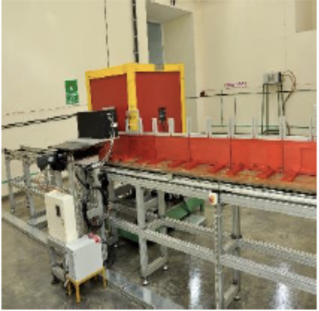
DAE – ISRO collaboration Portable 14 MeV neutron Generator surrounded by Moderator to get thermal Neutrons
